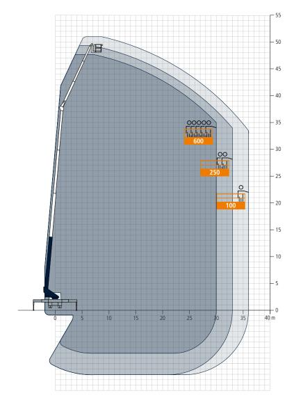
Two sections hydraulically extendible via remote control
